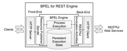
Fig. 6. Reference architecture for the BPEL for REST extensions.
