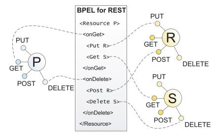
$\textbf{Fig. 1.} \ \ \text{Composing a RESTful Web service out of two existing ones using BPEL for REST.}$
