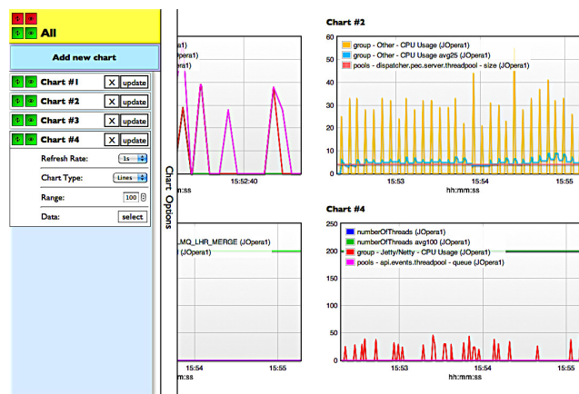
Figure 5. A screenshot of a real-time SOA monitor implemented using the Overseer framework.
