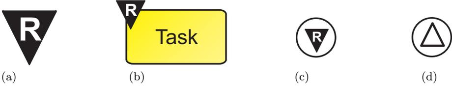
Fig. 3. The resource icon (a) applied to tasks published as a resource (b) and the new resource request event (c) which should be distinguished from the standard signal event (d)
