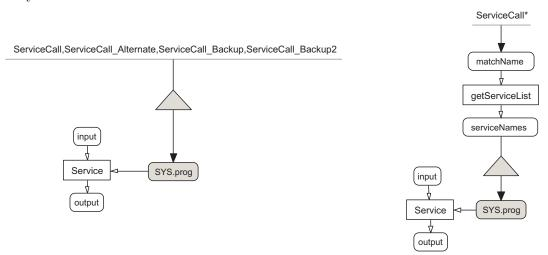
Figure 3.15.: Parallel invocation of alternative services This data flow graph represents the parallel invocation of the same four services of Figure 3.14. In the static implementation (left) the list of services is hard-coded, while in the dynamic implementation (right) the list of services is retrieved at runtime. The split operator can be configured so that the invocation will complete as soon as one of the services will respond successfully (Figure 3.16).
