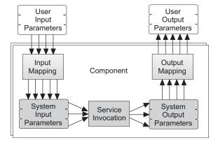
Figure 4.2.: Data flow mapping inside a component
