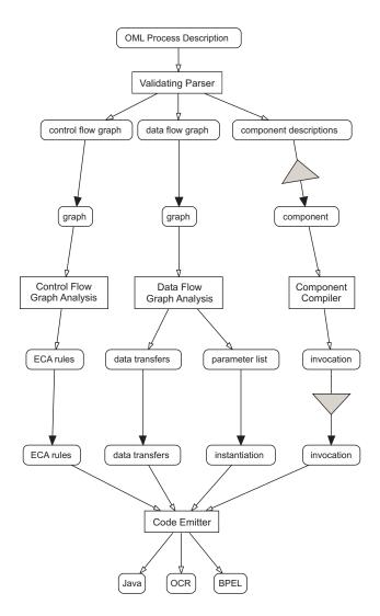
Figure 6.2.: Multi-stage architecture of the OML compiler
