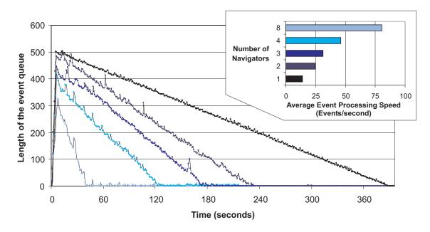
**Figure 8.8.:** Scalable navigation: event queue Behavior of the event queue with a fixed workload of 512 processes of 10 parallel tasks of 10 seconds and a variable number of parallel navigators.
