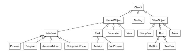
**Figure 5.4.:** Summary of the inheritance relationships between OML elements. This UML class diagram illustrates how the common attributes and the shared reference and aggregation relationships of the document elements have been structured in a single-inheritance tree. The Object, NamedObject, ViewObject, Box, Task and Interface elements are abstract and do not appear in an OML document.
