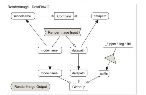
Figure 4.15.: Data flow view of the second part of the RenderImage process
