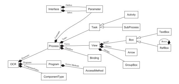
**Figure 5.3.:** Summary of the aggregation relationships between OML elements. For clarity also selected inheritance relationships to concrete classes have been included. This UML class diagram gives a good overview over the structure of an OML document. Starting from the Root (OCR) element, it shows where the other elements are located with respect to each other.
