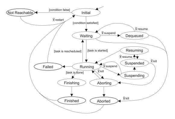
**Figure 6.8.:** Full state diagram of a task instance as it is followed by the code generated by the compiler
