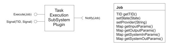
Figure 7.8.: Interface definition of the task execution subsystem The UML component diagram on the left defines the provided and required services of a task execution subsystem. The class diagram on the right defines the attributes of the Job interface, which is passed as a parameter to the task execution subsystem plugin.
