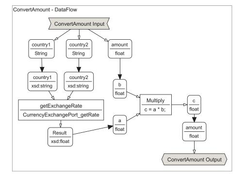
Figure 4.5.: Data flow view of the ConvertAmount process
