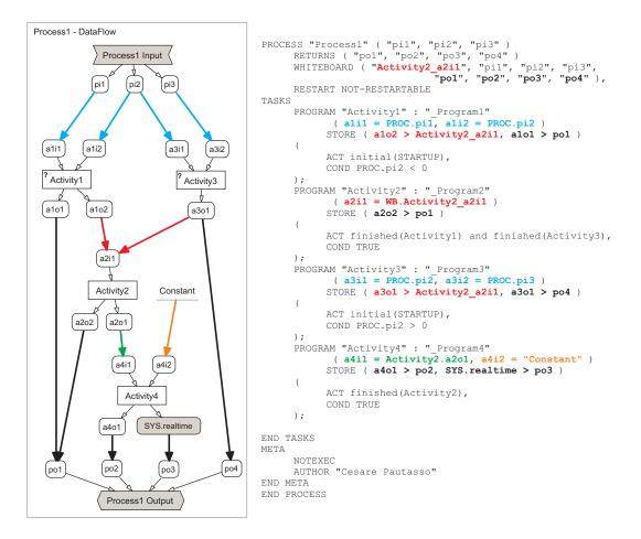
**Figure 6.3.:** Example showing a mapping from the JVCL visual syntax to the OCR textual syntax of a simple data flow graph of a process. (The intermediate OML representation is not shown)
