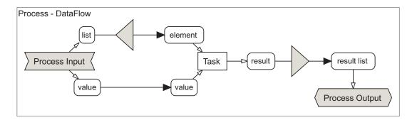
Figure 3.9.: Data flow syntax of the list-based loops
