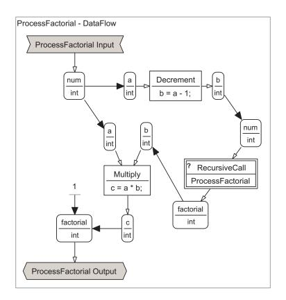
Figure 3.10.: Data flow view of a process to compute the factorial of an integer value
