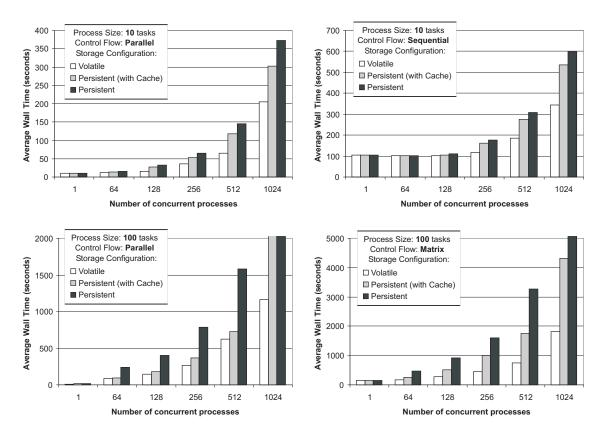
**Figure 8.3.:** Performance degradation of a centralized process support system under increasingly large workloads
