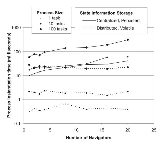
Figure 8.5.: Scalability of the process instantiation
