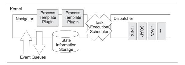
Figure 7.3.: Architecture of a Monolithic Process Execution Kernel
