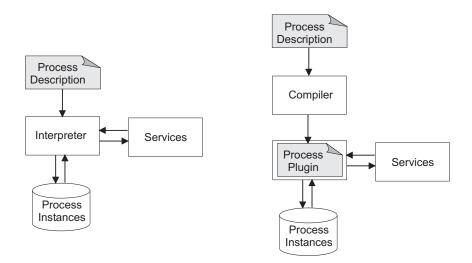
Figure 6.1.: Alternative approaches to process execution. In order to execute them, process descriptions can be either interpreted (left) or compiled (right).
