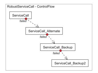
**Figure 3.14.:** Sequential invocation of alternative services This chain of four Service invocations is traversed as each call fails. JOpera attempts to contact the four alternative, equivalent services in the order specified by the control flow graph drawn by the developer.
