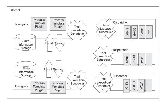
Figure 7.14.: Architecture of a Peer to Peer Process Execution Kernel
