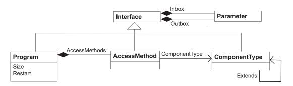
Figure 5.14.: Structure of the Program and Component type library.
