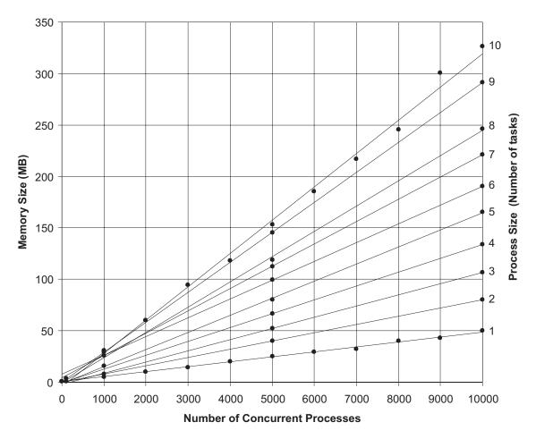
Figure 8.6.: Memory requirements for process instantiation
