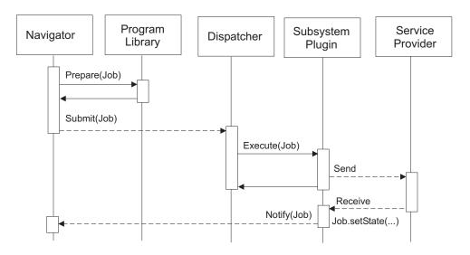
Figure 7.11.: Asynchronous service invocation
