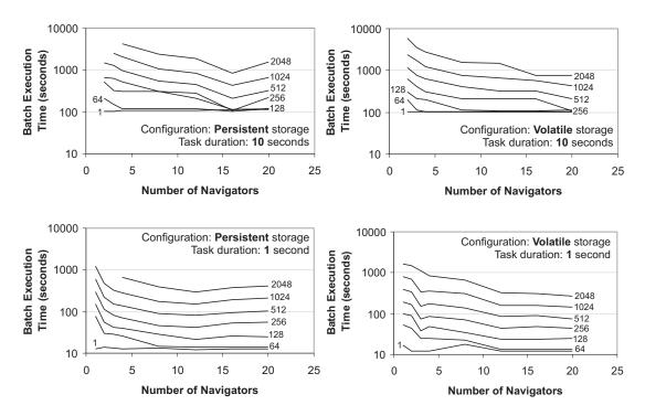
**Figure 8.9.:** Scalable navigation: batch execution time Execution time of batches processes having 10 tasks and sequential control flow topology as a function of 4 variables: 1) the number of navigators (X-Axis), the workload size (Z-Axis), the duration of the tasks and the system configuration (volatile or persistent storage)
