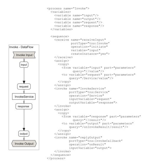
**Figure 6.4.:** A process with a single Web service invocation represented both in JVCL and in BPEL. The corresponding parts of the process are shown side by side.
