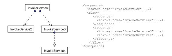
**Figure 6.5.:** A process invoking multiple Web services shown both in JVCL and in BPEL. There is a clear correspondence between the block-based structure of the BPEL representation and the control flow graph of the JVCL.
