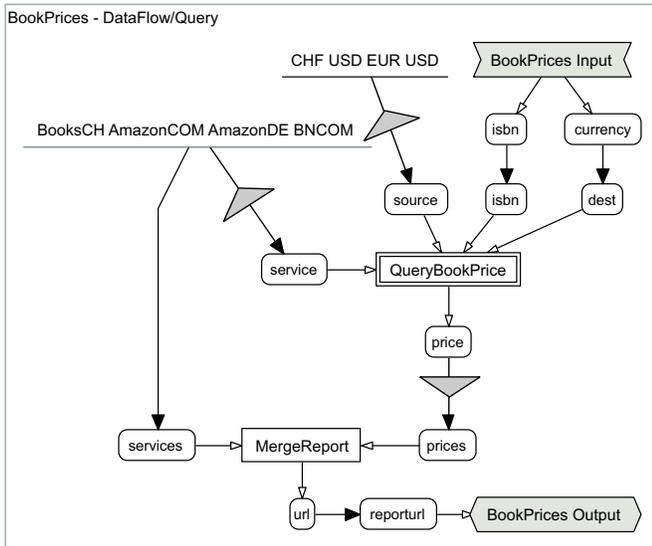
**Figure 8. Second data flow view of the BookPrices process with parallel split and merge operations**
