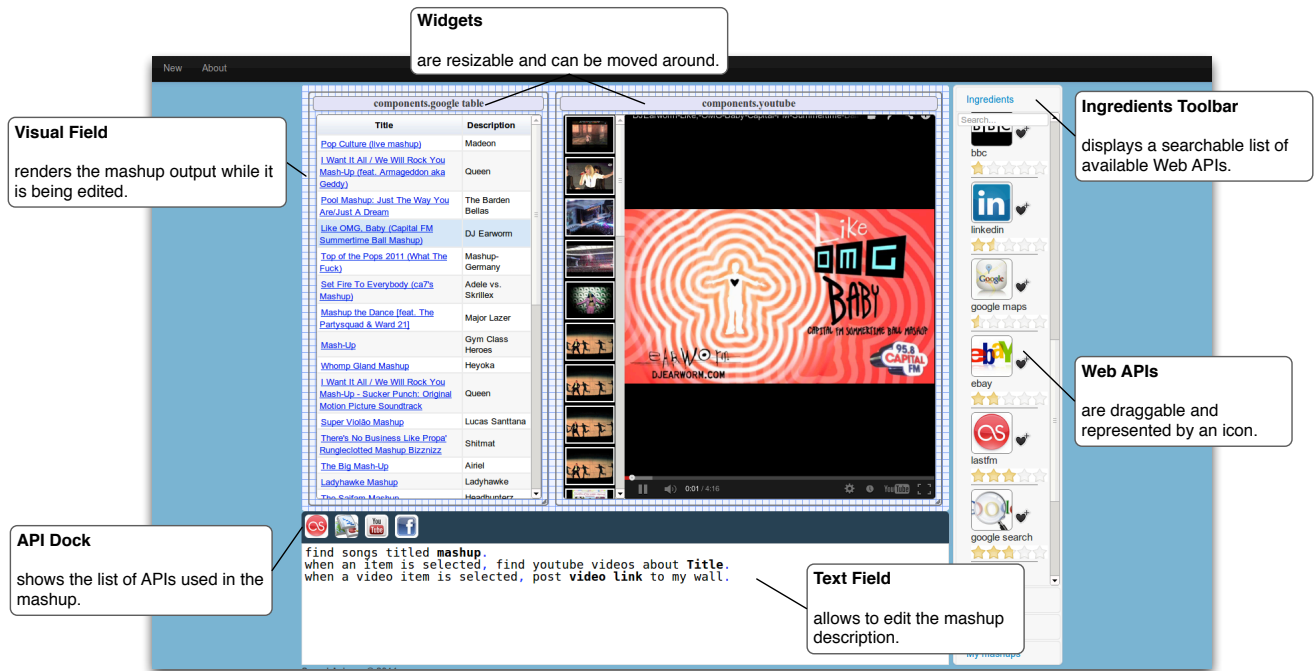
Fig. 1. NaturalMash environment: users type the description of the mashup in the text field and immediately see the output in the visual field. The output contains interactive widgets that can be resized and relocated. The ingredients toolbar helps with API discovery, while the dock gives a summary of the APIs used in the current mashup. Web APIs are abstracted away from the technologies they use and are represented as icon.
